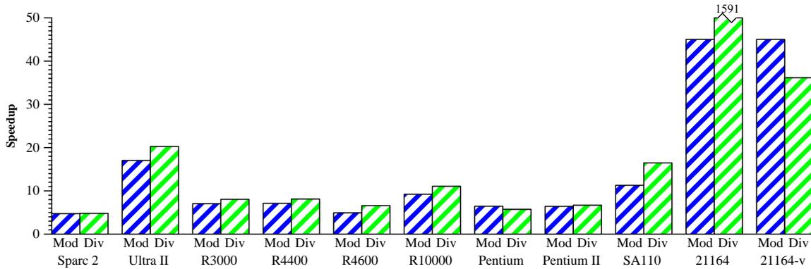
Figure 2: Performance improvement obtained with the strength reduction of modulo and division operations on several machines.
