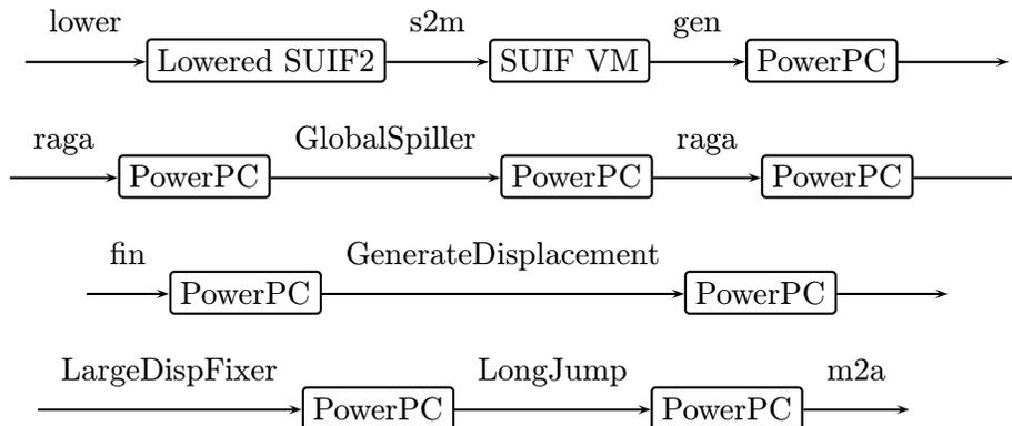
Figure 3.2: PowerPC compile chain detail
