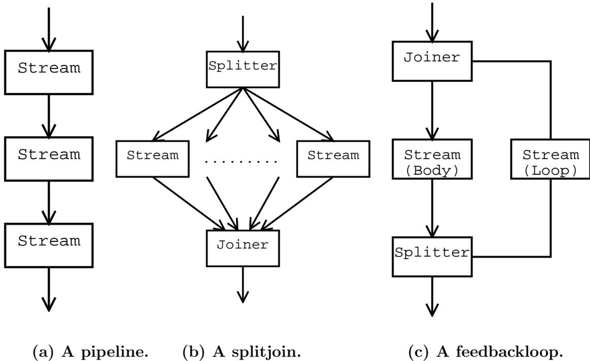
Figure 2-1: Container structures supported by StreamIt.
