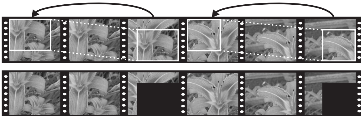
Figure 2-4: Eliminating temporal redundancy through forward motion estimation.
