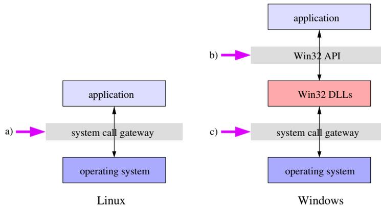
**Figure 2.** On Linux, the system call interface is the documented method of interacting with the operating system, as shown on the left. On Windows, however, a layer of user libraries makes up the Win32 API, which is the documented interface, while the system call layer is undocumented.
