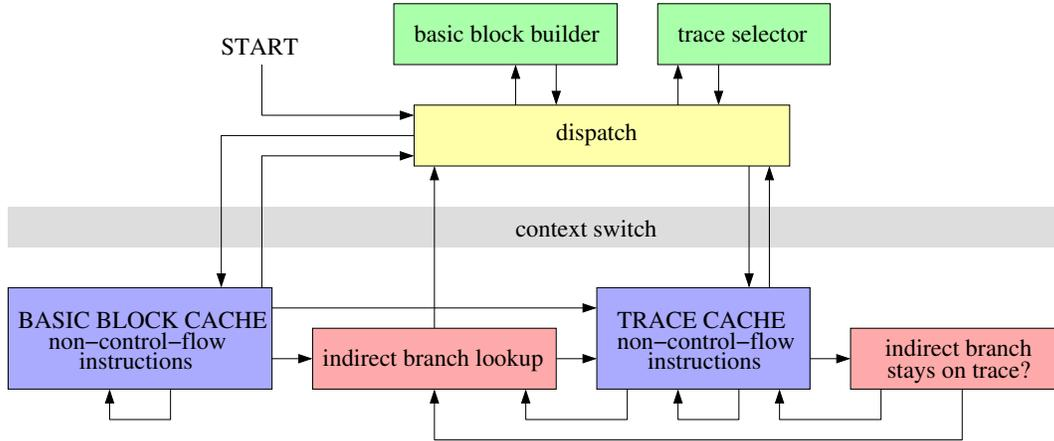
**Figure 1.** DynamoRIO system overview. A context switch separates the code cache (application state) from DynamoRIO code (system state); both execute in the same process and address space. Application code is copied into the two caches, with control transfers (shown by arrows in the figure) modified in order to retain control.
