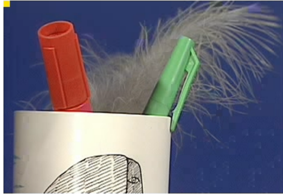
Figure A-3: An MPEG-2 rendered frame using memoization with untuned m distance ( m = 1000 ). SNR=45db from the source Figure A-1.
