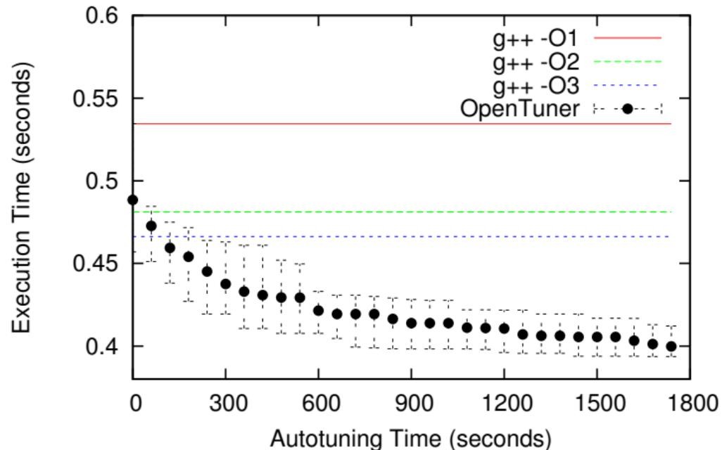
Autotune GCC flags for `tsp_ga.cpp`. Median of 30 runs, error bars are 20th and 80th percentiles.
