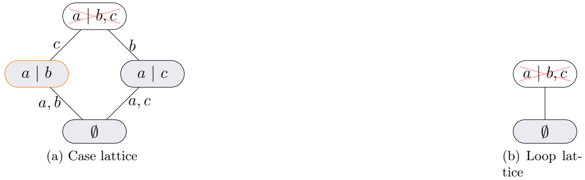
Figure 4-29: This example shows a case and a loop lattice for (a \cap b) \cup (a \cap c) - (a \cap b \cap c) . The highlighted lattice point denotes a special region. The code generator only needs to generate a loop over a , so when generating loops it is fine to use the lattice in (b). However, if attempting to generate cases within the loops using the lattice (b), the code generator lacks information saying it needs to perform a different computation in the highlight lattice point. It also has no way of knowing that it should not compute when a and c have defined values but not when all of a , b and c are defined. The case lattice in (a) contains all of this information and therefore this is the lattice that will be given to the code generator as input.
