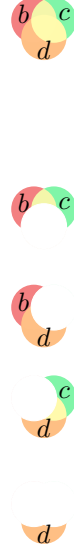
Figure 4-15: Iteration lattice and corresponding coiteration pseudocode for the iteration domain (b \cap c) \cup d . There is one while loop per lattice point and each while loop contains one if statement per sub-lattice point. Next to each while loop is a Venn diagrams showing the regions it coiterates over. The while loops iterate until a tensor in its region runs out of values, and the if statements check which region a coordinate is in. Depending on the region, different actions are taken.
