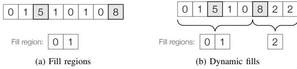
Fig. 5: Our generalization of fill values supports non-scalar fills (fill regions) and different fills for different parts of a tensor (dynamic fills).
